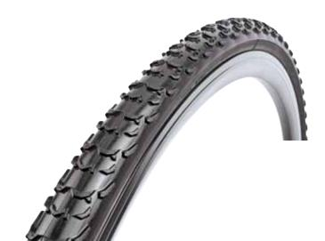
The third in Vittoria's family of cross racing tubulars, Cross Evo XM is for wet, muddy courses. Same 320 TPI casing, latex inner, and MTB World Cup-derived tread compound as other Cross Evos, but with aggressive, widely-spaced tread knobs to shed mud and grip firmly in acceleration, braking and cornering, even in the most challenging winter conditions.
