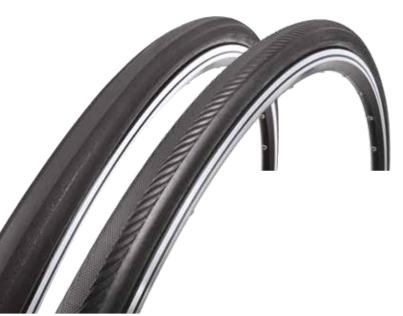
Unique reversible tire adapting to all conditions, 290 TPI Revo.KXS has Evo Slick racing tread on one face, Evo Tech wet-weather tread on the reverse. Puncture-resistant belt under each tread means double flat protection, yet still only 10% heavier than benchmark Corsa Evo.
