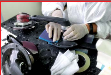
After moulding, the frame and its components are carefully sanded to go through the finishing stages.
