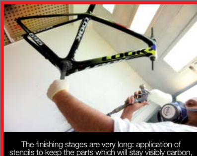
At LOOK, the carbon frames and accessories are made by hand. On average, around thirty hours are required to create one carbon frame.
