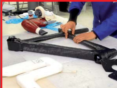
At LOOK, the carbon frames and accessories are made by hand. On average, around thirty hours are required to create one carbon frame.
