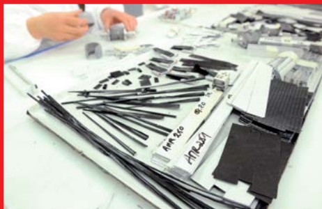
The creation of a carbon frame goes through an assembly stage of numerous pieces of carbon. For example, the 695 AEROLIGHT requires 508 pieces of carbon.
