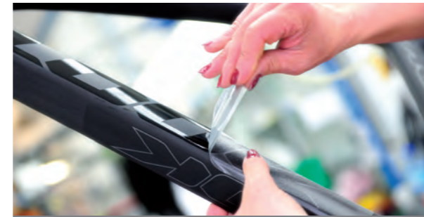
The finishing stages are very long: application of stencils to keep the parts which will stay visibly carbon, painting, anti-porousness testing, second stage of painting, removing stencils, adding decoration (transfers) and finally the application of the final varnish.
