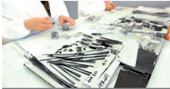
The creation of a carbon frame goes through an assembly stage of numerous pieces of carbon.
