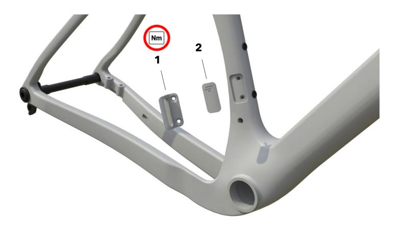
! Maximum torque for bolts: 4 Nm
